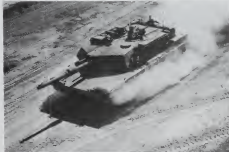
Figure 25: Modern heavy battle tanks. (Top) Soviet T-72, with 125-millimetre gun. A snorkel is mounted for submerged fording. (Middle) West German Leopard 2, with 120-millimetre gun. Smoke dischargers are fitted onto the side of the turret for concealment. (Bottom) U.S. M1A1, with 120-millimetre gun adapted from the Leopard 2. The M1A1 is powered by a gas turbine engine.
